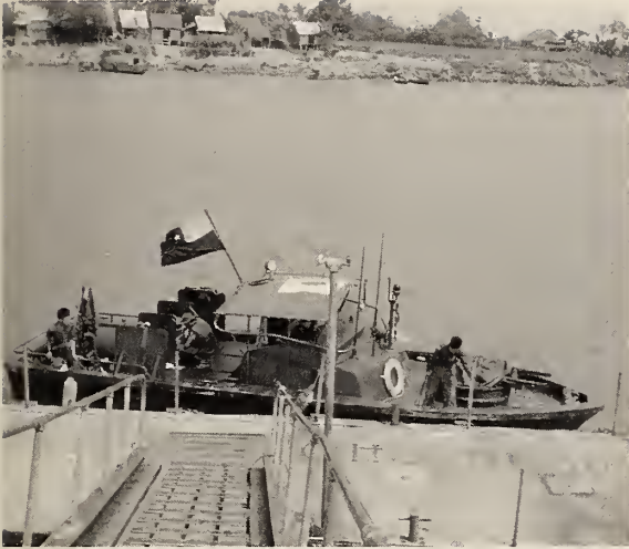
Photo courtesy of MajGen Donald R. Gardner, USMC Patrol craft were the essence of riverine operations. Here a Cambodian patrol boat riverine (PBR) docks at the Tan Chau base. This American-made craft used water-jet propulsion to operate in the shallow, restricted waterways. It is armed with Browning .50-caliber guns in the bow and M60 machine guns in the stern.
